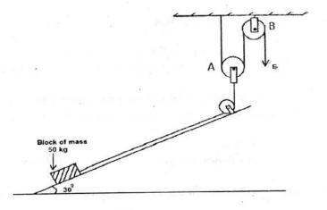
Refer to figure in question 55. Pulleys in the figure are massless and frictionless. Neglecting friction between 56) block and the ramp, the force that should be applied vertically downwards, at E, to slide the block along the ramp without acceleration is (g=10 m·s<sup>-1</sup>)
